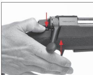
Press the bolt lock override button and lift the bolt handle.
