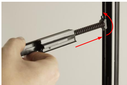
Figure E-2: Insert the rear of the bolt assembly into the stock rod channels
