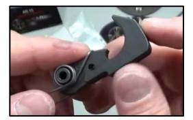
Step 10: Begin to Insert the Hammer back into the Lower.
