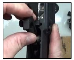
Step 11: Line up the Holes of the Spring and Reinstall the Hammer Hinge Pin. Make sure the Pin is even on both sides.
