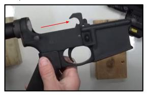
Step 6: Tap out the Hammer Hinge Pin. Keep your Punch Inserted.
