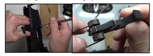
Step 8: Remove the Factory Hammer Spring from the Hammer.
