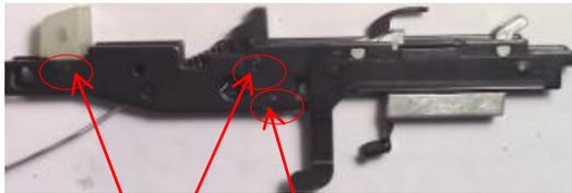
Step 17: Re-apply the 3 C-clips to the front plate.
