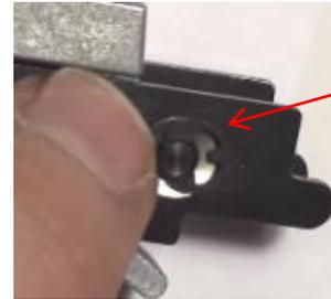
Step 16: Re-apply the washer and C-clip to the back plate.
