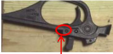
Step 1: Press out the forward pin on the trigger guard; from right to left or towards the red on the safety button
