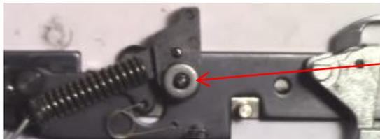
Step 11: Drop hammer back onto post on the plate. Make sure the notch drops into the hole on plate. Add gray spacer on top.
