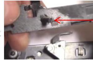
Step 14: Place the detent and spring into this hole on the other plate.
