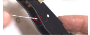
Step 4: Insert paper clip into small hole on hammer strut and release hammer.
