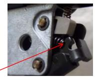
Step 5: Move the trigger into position and line up the holes to install the pin from the safety side.
