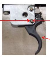
Step 3: Push the pin out; then remove the trigger and stock trigger return spring
