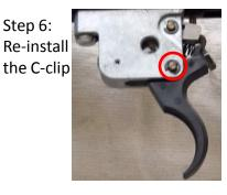
After you have reassembled your Marlin 900 Series make sure you do a function **check.** Cycle the action and load a snap cap or spent shell casing into the chamber. With the rifle safety on "safe" and the barrel pointed in a safe direction, verify that the rifle will not fire when you attempt to pull the trigger. Place the safety now on "fire" and now verify the hammer falls.
