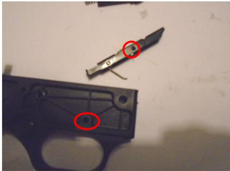
7. Drop the sear in so the end of the spring rests on the bottom of the housing like a ski. The right hole will have to line up with the trigger hinge pin hole. The spring has to be compressed to get it to line up. Then insert the pin. \*\*Note: If the spring rotates so the end is facing forward, it won't work.
