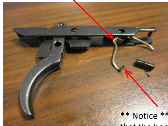
**\*\* Notice \*\*** Make sure that the hooked end is installed near the trigger and rests under the trigger hinge.
