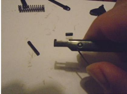
\*\* Once you have inserted the sear bar into the trigger housing you see the sear bar should rock when you pull the trigger. If it doesn't, the spring has rotated out of place.
