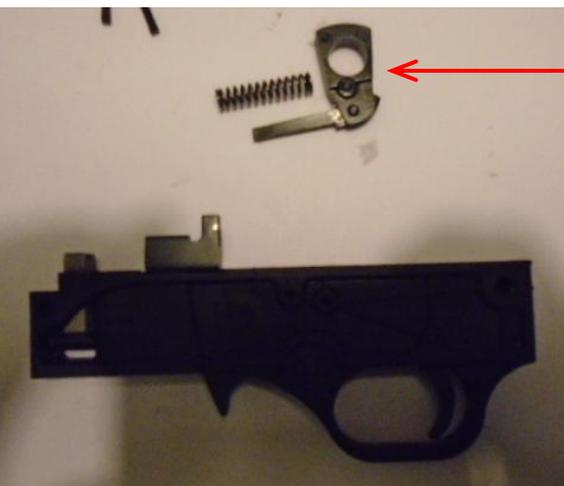
4. Remove hammer, spring and strut. The hinge pin is normally trapped between the sides of the housing. It will just fall out when removed.
